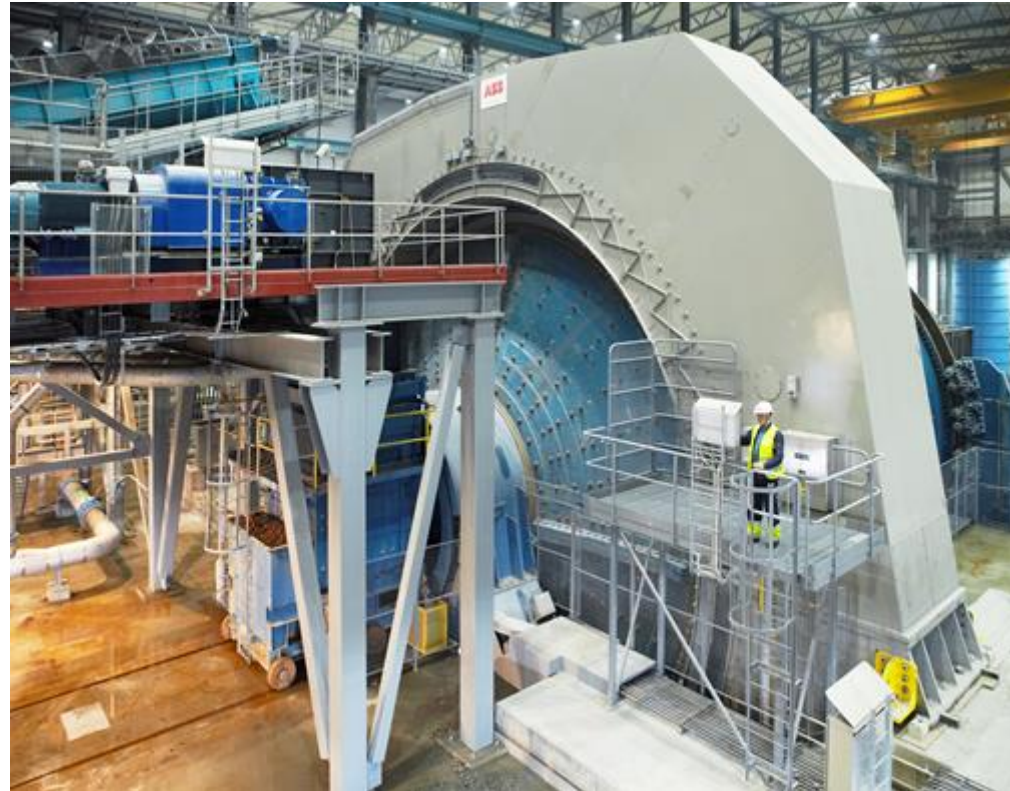
Pioneered by ABB in 1969 low rpm, high torque, diameter up to 12m, up to ~30MW
